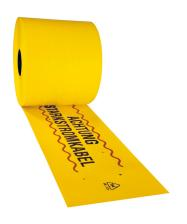
Cable protection tape no 09 was developed to complement no 08 and, thanks to its perforation, allows the passage of humidity, thus preventing unwanted build-up of heat. This version is produced in material thicknesses of 0.55 mm and 1.0 mm.
