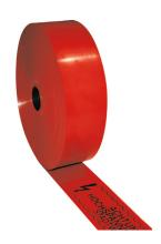
Type No 08 is certified to DIN 54841-5 and suitable for the most common areas of application. This version in thicknesses of between 1.5 mm and 4 mm also passes the mandatory dart drop impact test, which simulates the damage potentially caused by spades, pickaxes and sharp-edged filling material.
