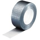
Technical features Material: PE sheet with woven cloth inlay, rubber-based adhesive, PVC-free Colour: silver-grey Properties: easy to tear off by hand, great adhesive strength, repels splash water
